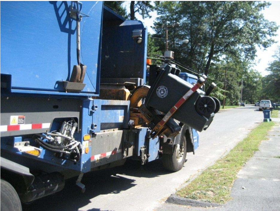
The mechanical arm of a new automated trash truck lifts a refuse container on collection day in Bedford.
